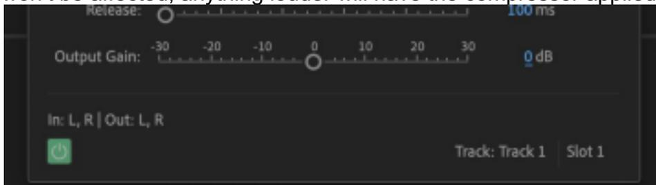
Ratio: The higher the ratio the more severe the compression. Attack and Release are ways to smooth the compression's effect. Attack leads up to the signal and how it gradually turns the compressor off is release.
