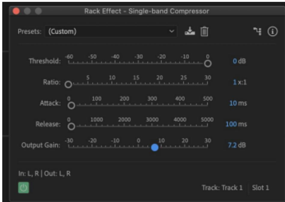
Notice in the image how the Output gain was raised by 7.2db, that is not always the case, you will want to increase it only when needed.
